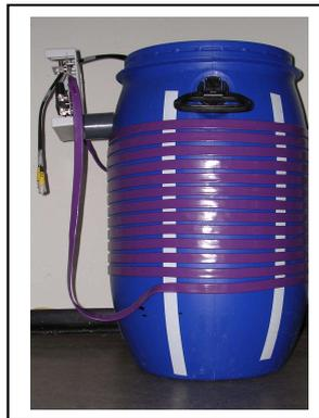
Figure 7 External coil with class E driver
