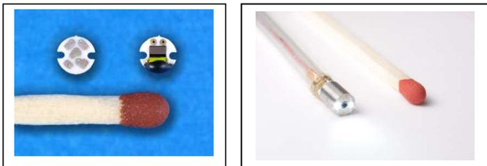
Figure 3 Ceramic board with IVP1 image sensor and pad connectors (left), IVP1 videoprobe head with optics and illumination (right)
